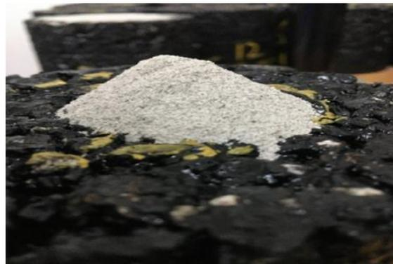
Fig. (4). The volume of sand vs sample.
