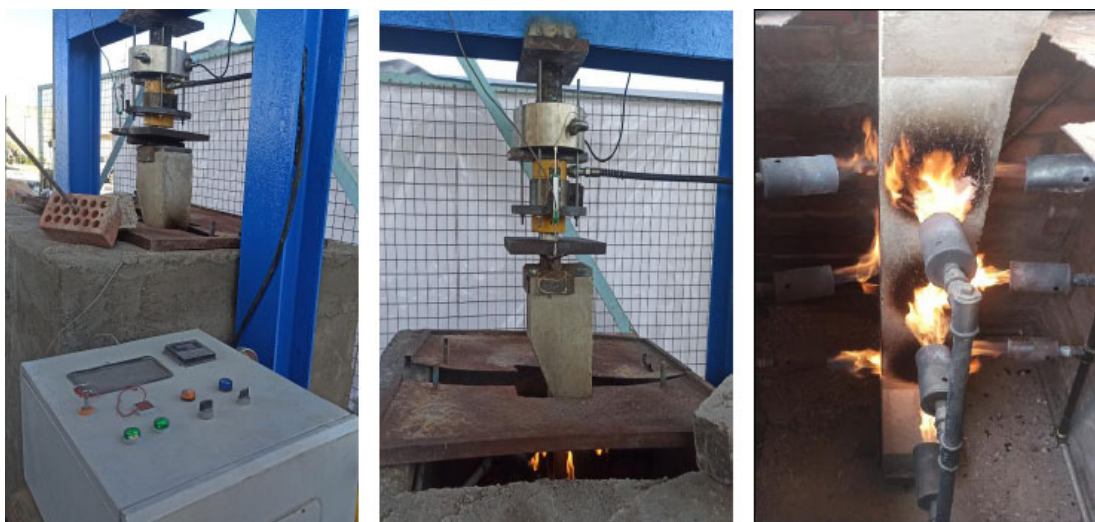
Fig. (4). Specimens subjected to fire exposure under pre-loading curve.
