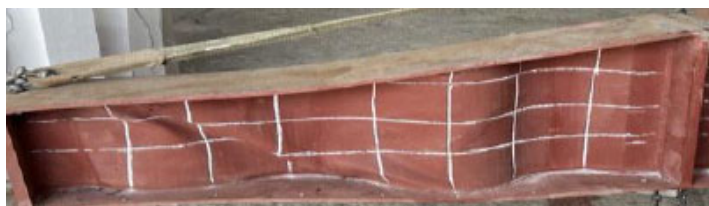
Fig. (6). Buckling pattern observed in TSW400 under 3-point loading.
