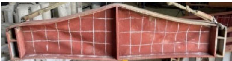
Fig. (7). Buckling pattern observed in TFW400 under 3-point loading [first published in Asian Journal of Civil Engineering, vol. 26, pp. 2837-2851, 2025, Springer Nature].
