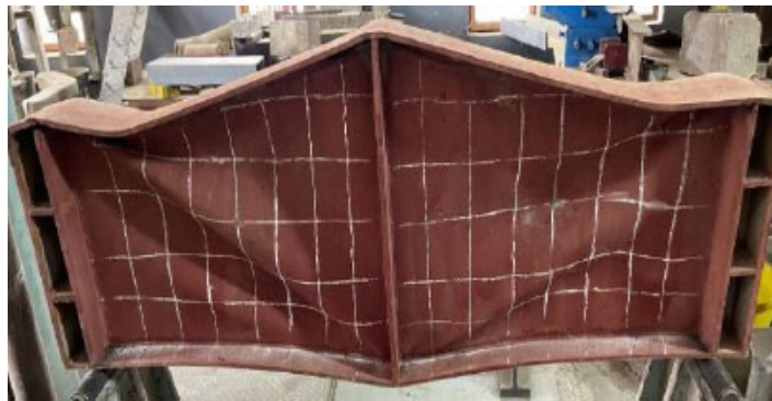
Fig. (9). Buckling pattern observed in TFW600 under 3-point loading [first published in Asian Journal of Civil Engineering, vol. 26, pp. 2837-2851, 2025, Springer Nature].
