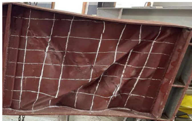
Fig. (10). Buckling pattern observed in TSW800 under 3-point loading.
