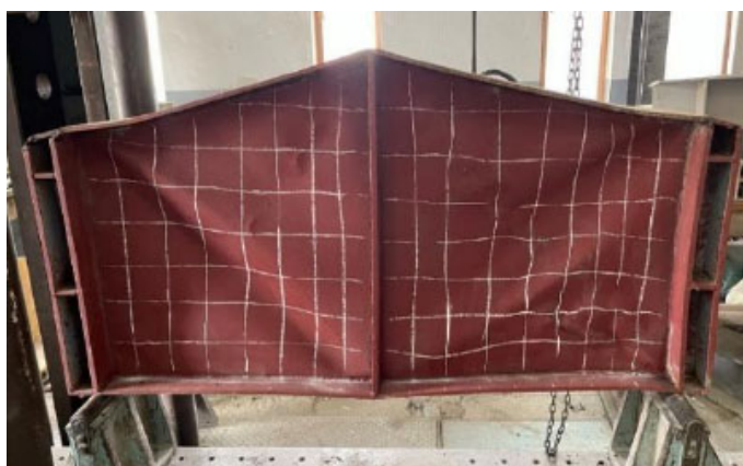
Fig. (11). Buckling pattern observed in TFW800 under 3-point loading.
