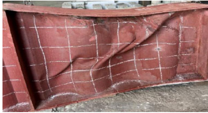
Fig. (8). Buckling pattern observed in TSW600 under 3-point loading.
